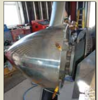
Booted Clecos prevent scratching the nice new spun-aluminum dome during installation.
