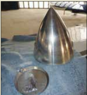
The finished job—it took about three hours of work to mount this on the existing rear bulkhead. It would take a few more hours if you needed a new rear plate.
