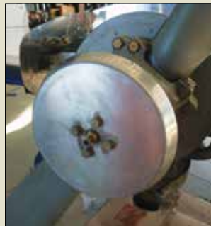
The new forward bulkhead is pre-drilled for the hub mounting screws. Measuring and drilling the flange for nutplates was fairly simple. (Note that the bolts were not yet safetied in this picture.)
