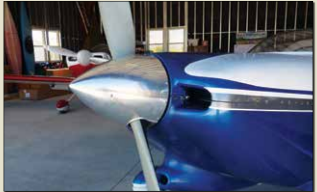
The finished job—it took about three hours of work to mount this on the existing rear bulkhead. It would take a few more hours if you needed a new rear plate.
